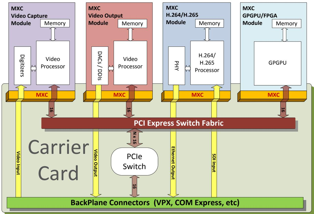
Figure 2: MXC cards intercommunicate over PCI Express, creating an advanced, high speed, video solution.
