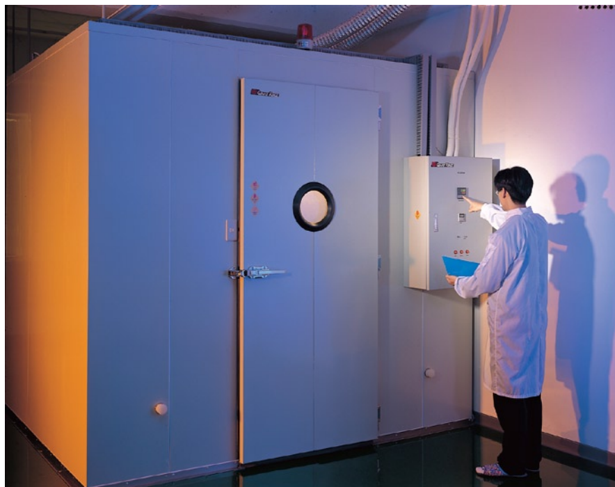
Extended Temperature Testing verifies that all boards will operate and function at temperatures from -40^{\circ} to +85^{\circ}\text{C} or other ranges.
