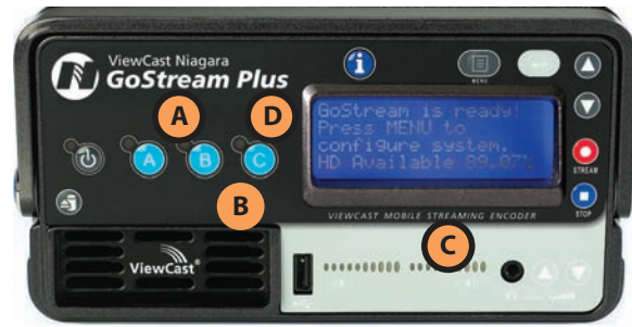
Pre-defined encoder options allow streaming to begin with the push of a button.
