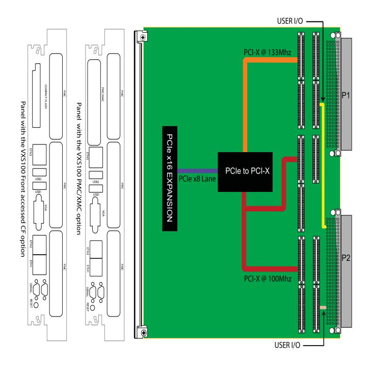
FIGURE 1. VXS102 Functional Block Diagram
