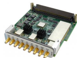
FMC229 Quad DAC 16-bit 2.8 GSPS
