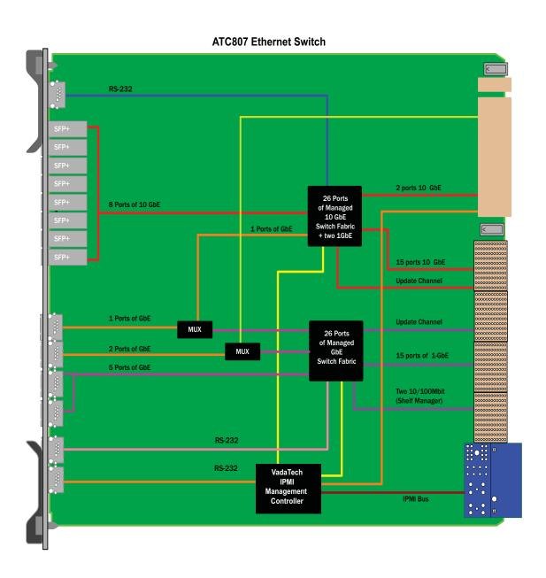
FIGURE 1. ATC807 Functional Block Diagram
