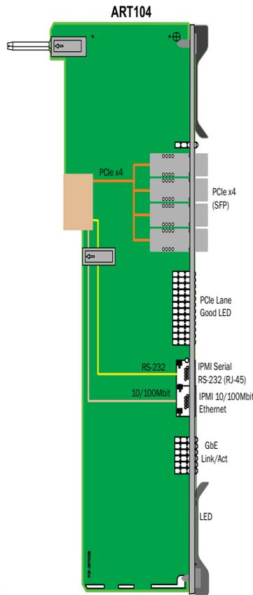
**FIGURE 1.** ART104 Functional Block Diagram
