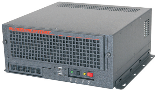
Trenton TVC3400 Shelfmount / Wallmount Video Controller Shown with a MicroATX motherboard
