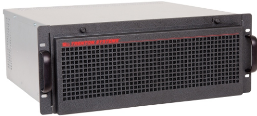
Trenton TTX4100 PCIe Expansion Chassis Shown with a x16 PCIe target card and backplane
