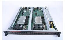
**Lightweight Construction** The TRC1001 features a chassis constructed with rugged yet lightweight aluminum.
