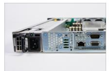
**1200W Removable PSU** Ample wattage in a low-profile power supply that easily supports both processor boards.
