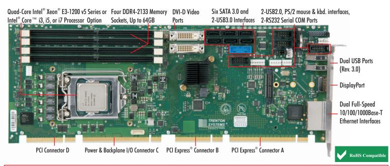
Trenton's TKL8255 single board computer delivers the performance of Intel Xeon E3-1200 v6 series processors to the PICMG 1.3 standard. Leveraging advanced peripheral interconnect topologies and multimedia interfaces, the TKL8255 ensures PICMG 1.3-based systems will outperform for years to come while maintaining legacy compatibility. All-digital display interfaces for graphically-intensive applications
