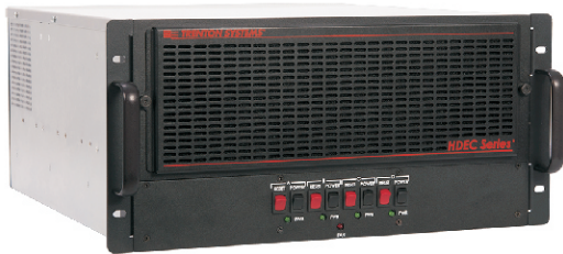
THS5091 HDEC Series Rackmount Computer Shown with a four-segment backplane and four SHBs
