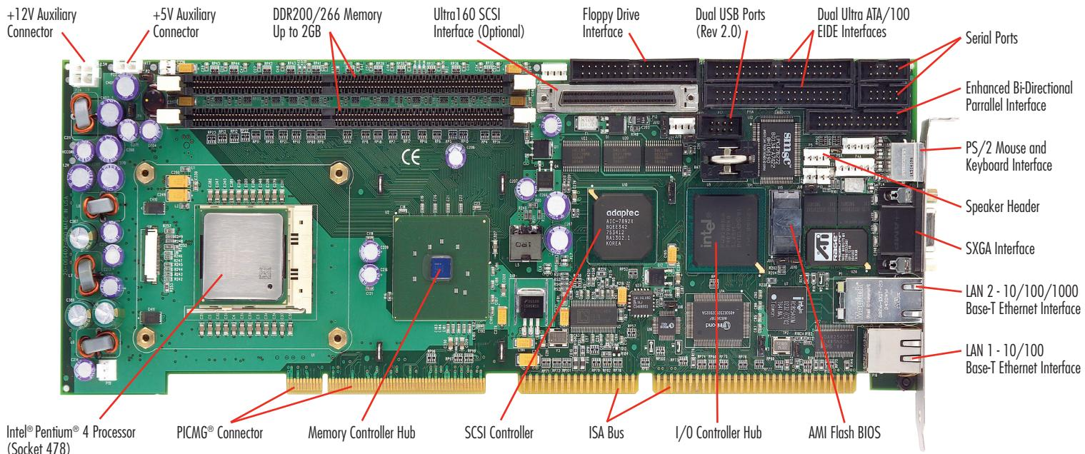
**The T4R is a single board computer specifically designed to bring high-performance processing to legacy applications. The power-control circuitry on the T4R has been engineered to accommodate older backplanes and power supply harness designs. Enhanced video memory and drop-in SBC replacement capability enable cost-effective embedded computing system upgrades.**
