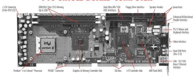
The T4G provides a base level of functionality and value required in less demanding single board computer applications. Economical innovations like the Intel® 845GV chipset, with integrated graphics and video, combine with Pentium® 4 and Celeron® processor options to maximize system value in low-end applications. Trenton's renowned SBC quality, longevity and dependability are standard features on the T4G.
