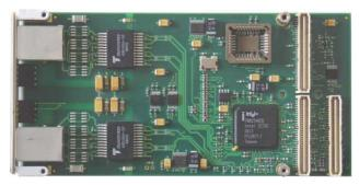
An Intel™ 82546EB Ethernet Controller (Intel™ 82546GB for ROHS compliant version) is used, which supports 10, 100 and 1000 Mbit/s transmission rates for half and full duplex operation. The TPMC884 is capable of performing an auto negotiation algorithm which allows both linkpartners to find out the best link-parameters by themselves. The TPMC884 is widely user configurable via configuration and status register access over the PCI bus. Front panel mounted LEDs indicate various network activities.
