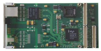
An Intel™ 82545EM Ethernet Controller (82545GM for RoHS compliant product) is used, which supports 10, 100 and 1000 Mbit/s transmission rates for half and full duplex operation. The TPMC883 is capable of performing an auto negotiation algorithm which allows both link-partners to find out the best link-parameters by themselves. The TPMC883 is widely user configurable via configuration and status register access over the PCI bus. Front panel mounted LEDs indicate various network activities.
