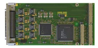
The TPMC862 provides front panel I/O via a HD68 SCSI-3 type connector and rear I/O via P14.
