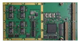
The serial communication controller is implemented in FPGA logic, along with the bus master capable PCI interface, guaranteeing long term availability and having the option to implement additional functions in the future.
