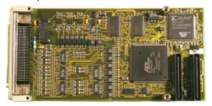
An 'auto reference mode' provides the possibility of automatic preload of the encoder counter during normal operation, whenever the motion system passes the reference position.
