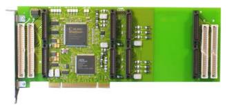
The IP power lines are fuse protected by self healing fuses and RF filtered. The operating temperature range is -40°C to +85°C.
