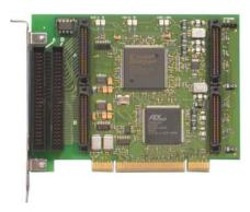
The IP power lines are fuse protected by self healing fuses and RF filtered. The operating temperature range is -40°C to +85°C.
