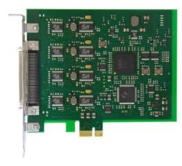
Each channel has a receive and a transmit FIFO of 512 long words (32 bit) per channel for high data throughput.
