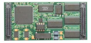
An interrupt can be generated at end-of-settling, end-ofconversion or end-of-sequencer cycle supporting an 8 bit vector.
