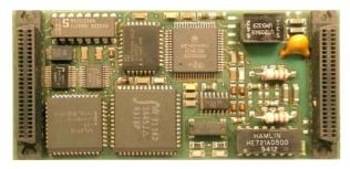
The communication is executed via a 4 Kbyte Dual Port RAM. A 32 Kbyte EPROM is used to store the protocol firmware of the NEURON Chip 3150 and the application program. All modules have a PROM with the protocol firmware and the MIP/DPR host interface software preinstalled.
