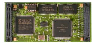
The TIP302 provides 1 Mbytes of static RAM (SRAM) as dual-port memory for both, MC68302 code and user data. The code is downloaded to the SRAM by the IP host CPU prior to removing the MC68302 reset signal by writing to a control register. Once the MC68302 reset signal is removed, the MC68302 starts fetching code from the SRAM.
