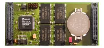
Four 512 Kbit x eight low power SRAM devices are used to provide two banks of 1 Mbyte (16 bit wide) SRAM memory.
