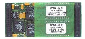
Two converter accuracies are available: TIP150-x0x with 4 arcmin +1LSB and TIP150-x1x with 2 arcmin +1LSB. The customer specific signal conditioning adapter (TIP150-Ayxx) per channel provides an easy interface to the different types of synchro and resolvers. For highest accuracy the on board reference oscillator of the signal conditioning adapter TIP150-A2-xx and TIP150-A4-xx automatically compensates the phase error generated by the synchro / resolver.
