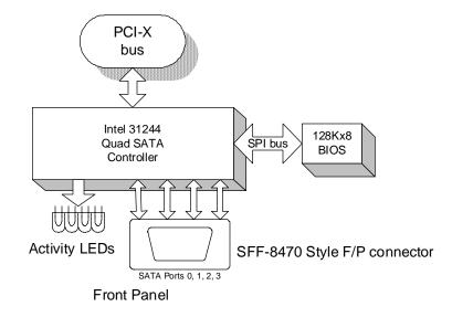
The Serial ATA controller provides four 1.5Gb per second links on a PMC front panel by using a Small Form Factor 8470 connector as specified in the SATA II connector standard. This connector provides a robust connection to a 4-lane SATA cable using screwlocks and jackscrews to secure the cable to the PMC front panel connector.
