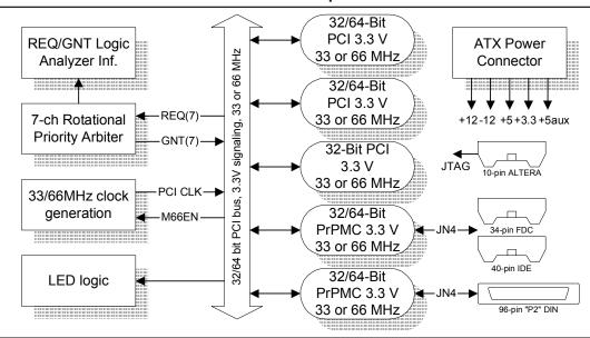
The FlexATX Development Platform provides two PrPMC and three edge-finger PCI bus slots in a standard 9"x7.5" form-factor used in Personal ComputerATX enclosures.
