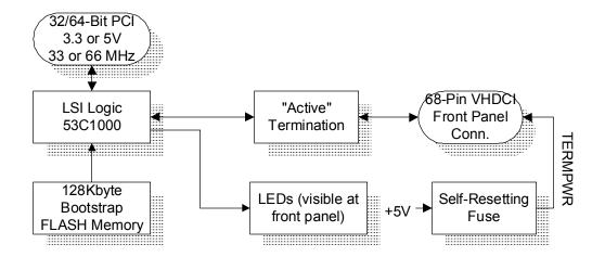
The ULTRA160 SCSI PMC adapter interfaces a host board PCI bus to a standard SCSI interface via an LSI Logic 53C1000 controller for operation with single ended or Low-Voltage Differential signaling.
