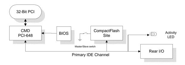
The Front Panel CompactFlash Adapter, when mated to a host or carrier card, provides an interface between the PCI bus and a CompactFlash device (Type I or II) mounted on the Adapter. The Adapter also can interface other IDE/ATA devices, via its rear I/O connector (PN4) on the Adapter.
