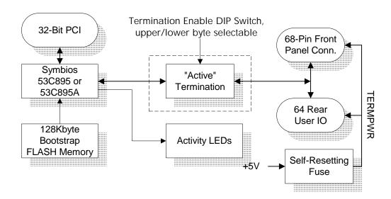
The ULTRA2 SCSI PMC adapter interfaces a host board PCI bus to a standard SCSI interface via either a Symbios 53C895 or 53C895A controller for operation with single ended or Low-Voltage Differential signaling.
