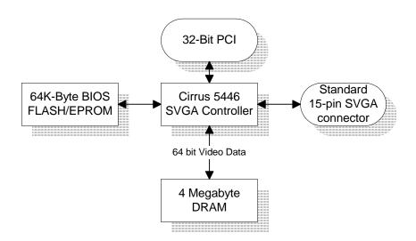
The Technobox Super Video Graphics Array (SVGA) Adapter PMC implements a standard graphics controller similar to graphics controllers found in Personal Computer applications.
