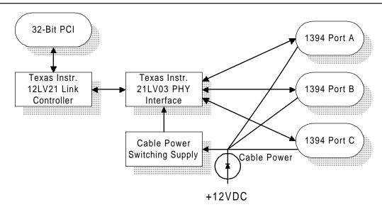
The IEEE P1394 PMC from Technobox provides 100 Mb/s and 200 Mb/s 1394 serial bus interface with connectivity for up to three 1394 ports.
