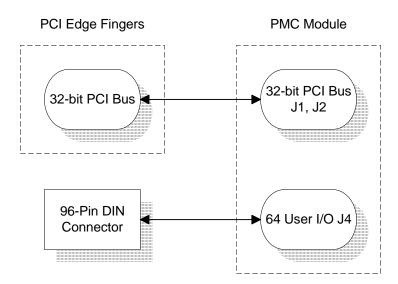
This PMC to PCI Adapter product from Technobox permits delivery of PMC-derived applications in a standard PCI environment.
