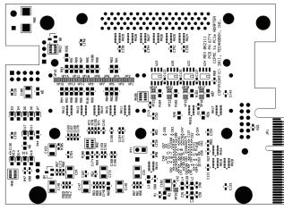
the PEX8114 bridge is a four lane (4X) generation 1 PCI Express interface. The PCI/PCI-X secondary side operates at 33, 50, 66, 100 or 133 MHz in 32 or 64 bit bus width mode. Use of 5V only PCI signaling ccPMC cards is prevented by voltage keying.
