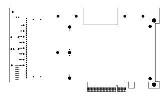
This board has been carefully designed to minimize signal lengths on the 2.5GHz LVDS PCI Express bus. Four impedance-controlled signal layers and four power planes (2xGND, 3.3V, and V1.0) are employed to minimize transmission line effects. A high quality 2.5 mm thick
