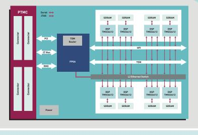
The SurfRider-812/PTMC is a PMC/PTMC mezzanine card that can be mounted on top of a PCI, cPCI or ATCA blade.
