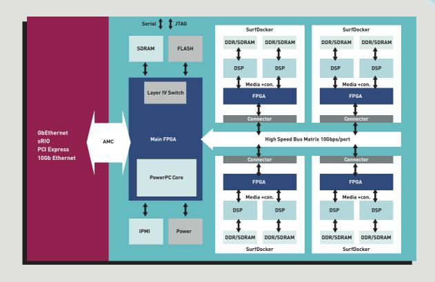
Surf's SurfRider/AMC solution is comprised of a main board and SurfDocker plug-in modules, enabling exceptional flexibility and comprehensive management and control of all components.
