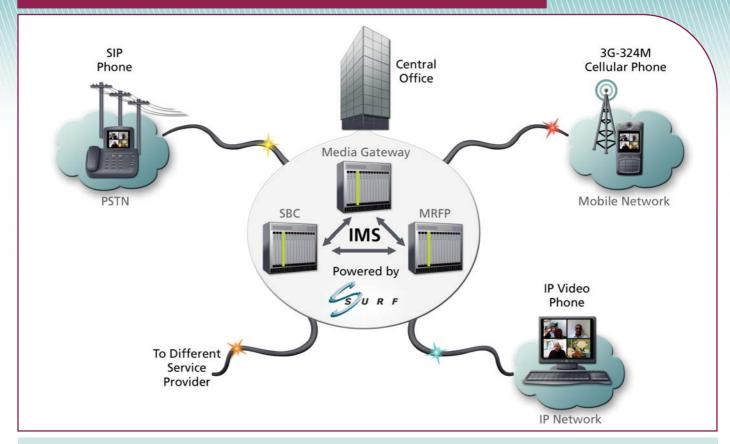
Typical network topology illustrating how the SurfRider/AMC DSP resource card integrates into network infrastructure equipment to enable convergence of Voice + Video + Data across Wireline and Wireless networks.
