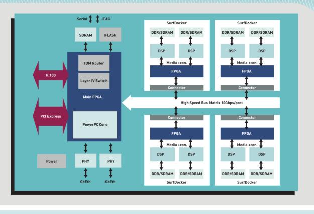
Surf's SurfExpress/PCIe solution is comprised of a main board and plug-in modules, enabling exceptional flexibility and comprehensive management and control of all components.
