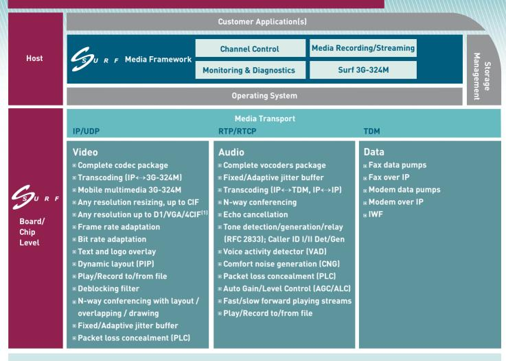
The system architecture used in the SurfExpress/PCIe is optimized to reduce bottlenecks.
