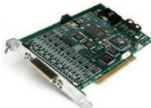
Swift PCI NTDS Parallel A/B/C/H with 120-pin connector
