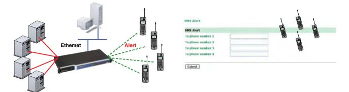
The NM-GPRS/GSM module provides the NPort 6000 device server with an SMS Alert function. NPort 6000 device servers support up to 4 phone numbers that can be configured to receive alert messages. As shown in the following table, there are four event categories (System, Network, Configure, Serial Port), and a total of eight different options that can be configured.
