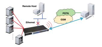
connection failure has occurred, data from the serial device will be sent out through the GSM/GPRS network. When the remote host on the Ethernet side returns to normal status, data will again be sent through the Ethernet connection. The NPort 6000 backup function makes your data transmission safer and more reliable.
