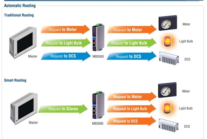
The MGate™ MB3270, MB3280, and MB3480 include smart routing for enhanced compatibility with existing Modbus networks. Other Modbus gateways require a separate socket connection for each serial port, making them useless for TCP masters that can only open one connection. With smart routing on the MB3000 Modbus gateway, a TCP master can use just one socket connection to command serial slaves on every serial port.
