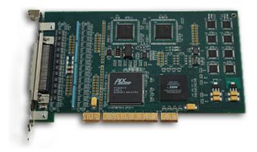
The PCI-SI04B board is a four channel serial interface card which provides high speed, full-duplex, multi-protocol serial capability for PCI applications. The PCI-SIO4B combines two multi-protocol Dual Universal Serial Controllers (USC®) and 8 external FIFOs to provide four fully independent asynchronous or synchronous RS422/RS485 serial channels. These features, along with a high performance PCI interface engine, give the PCI-SIO4B unsurpassed performance in a serial interface card.
