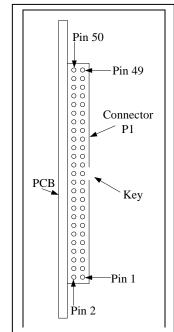
The connector mounted on the board is manufactured by Tyco and has the part number AMP 1-103311-0. The part number of the mating connector is AMP 1-746285.
