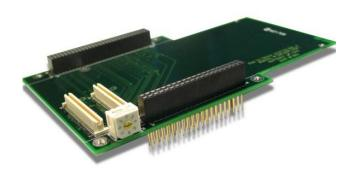
The PMC-to-PC/104-Plus Adapter accommodates one PMC Card to a PC/104-Plus environment. The adapter is stackable and can be used with multiple devices.
