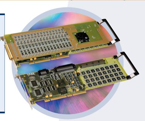
Continuing the evolution of the ICS-645 high-speed acoustic product line, the new ICS-645D brings a comprehensive suite of data acquisition capabilities to industrial PC systems. Combining high-speed oversampled ADCs (AD9260) with onboard gain and filtering, as well as high-speed data routes (PCI 64/66 or FPDP II) back to the host system, the board has been optimized to provide maximum functionality in a single full length PCI card.
