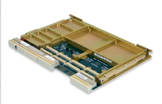
**DCPMC64** is a rugged Dual CompactPCI 64-bit PMC (DCPMC64) carrier module in 6U form factor that can accommodated two PMC modules for increasing I/O capability to a system.
