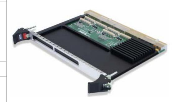
**DCPMC** is a Dual Compact PCI Mezzanine Card (DCPMC)—a conduction-cooled carrier card in a 6U form factor that can accommodate two PMC modules for adding or increasing I/O capability to a system. It can connect two PMC modules to any standard CompactPCI backplane through a 32-bit 33MHz cPCI bus. The DCPMC implements the 21152 PCI/PCI Bridge to data transactions from the PCI bus (system host) to two standard PMC sites.
