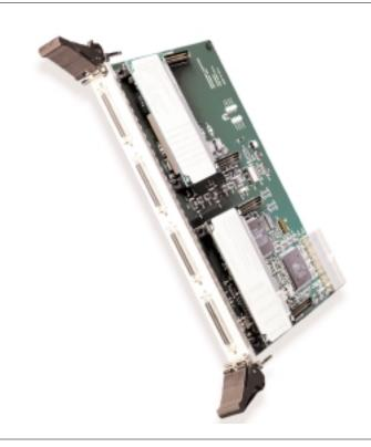
**SBS' CPCI-200A IndustryPack carrier board** provides four IndustryPack slots on a 6U CompactPCI card. Two versions are available: the CPCI-200A-FP provides shielded 50-pin SCSI2-style front panel connectors for IndustryPack I/O; the CPCI-200A-BP provides IndustryPack I/O via the CompactPCI J4 and J5 connectors. Rear panel transition modules, BIO-3 and BIO-4, are available from SBS.
